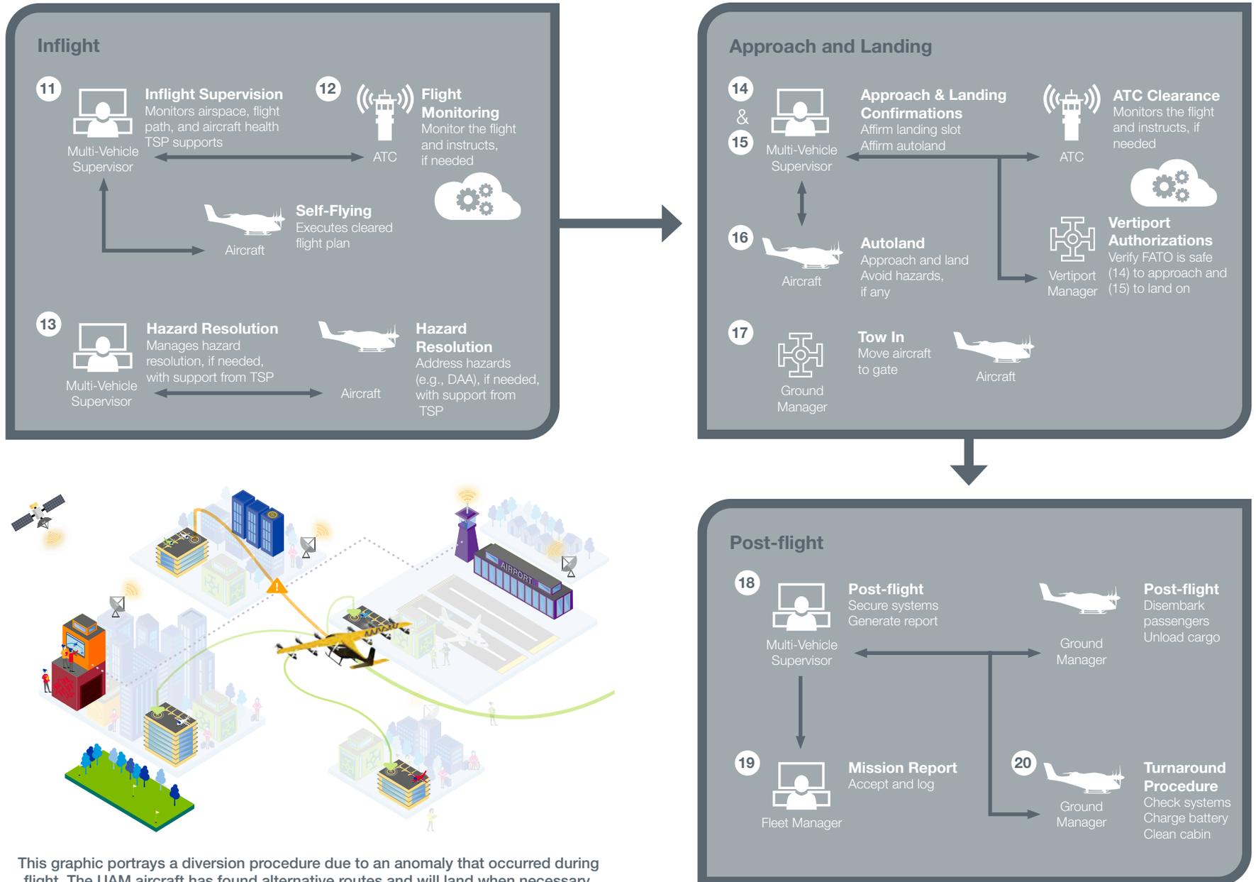
This graphic portrays a diversion procedure due to an anomaly that occurred during flight. The UAM aircraft has found alternative routes and will land when necessary.
