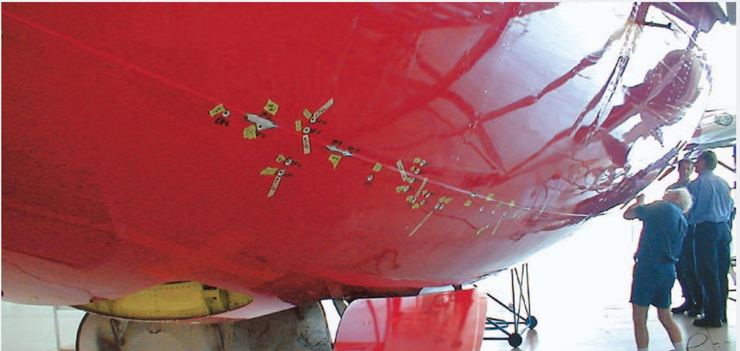
lightning strike is damage caused to bonding straps. These straps can become crushed during a lightning strike due to the high electromagnetic forces.
