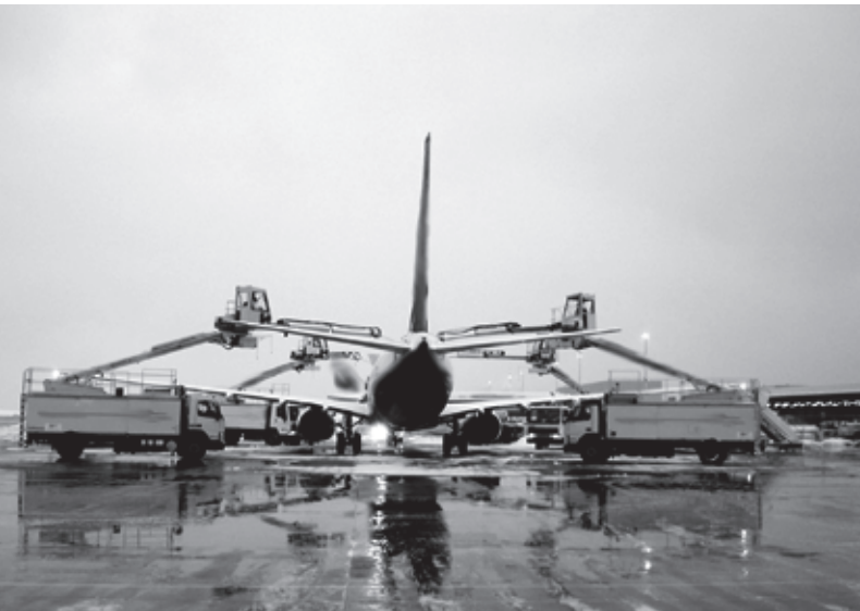
Large volumes of deicing/anti-icing fluids are commonly used during severe winter weather, especially on small- and medium-sized airplanes.
