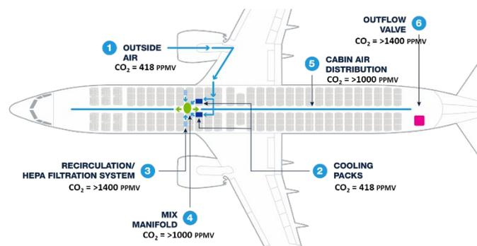
Figure 1: Carbon dioxide concentrations by location in commercial airplanes
