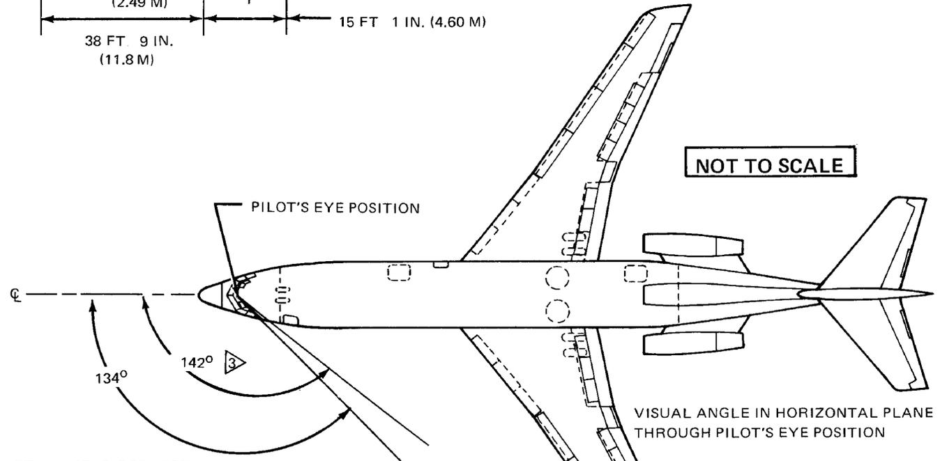
NOTE: HEAD ROTATED ABOUT POINT 3.3 IN. (0.08 M) AFT OF PILOT'S EYE POSITION
