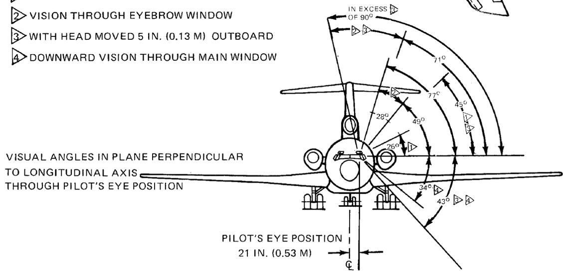
**4.4 VISIBILITY FROM COCKPIT IN STATIC POSITION (AMBINOcular VISION) MODEL 727-100**
