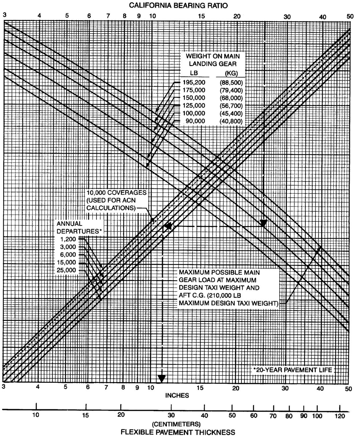
**7.5.1 FLEXIBLE PAVEMENT REQUIREMENTS—U.S. ARMY CORPS OF ENGINEERS DESIGN METHOD (S-77-1) AND F.A.A. DESIGN METHOD MODEL 727**
