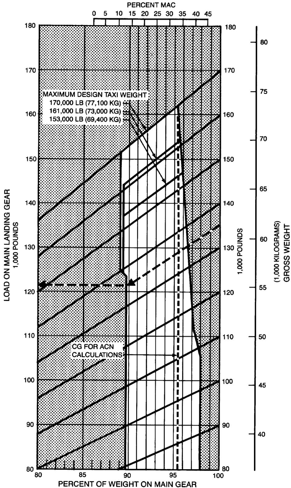
**7.4.1 LANDING GEAR LOADING ON PAVEMENT**
