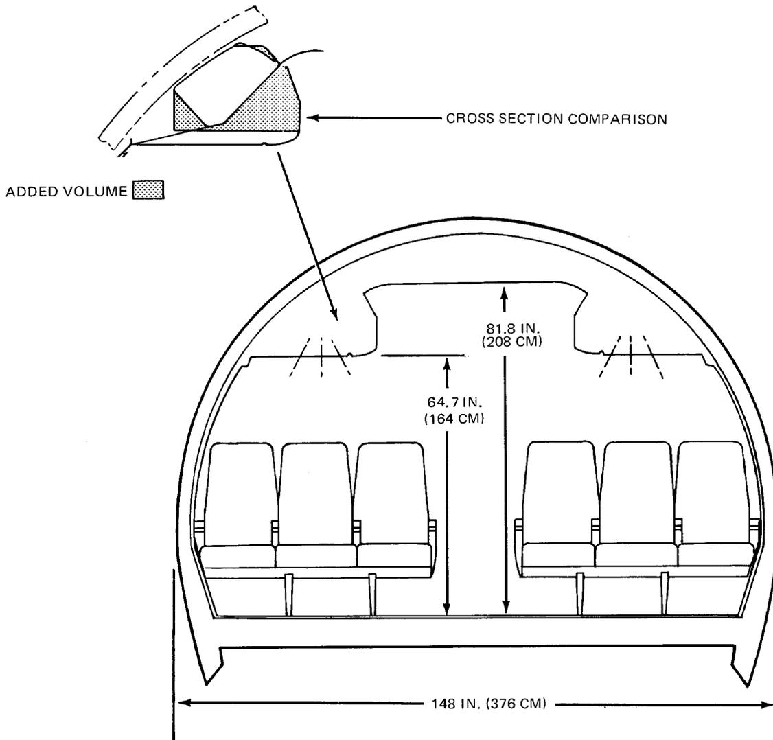
INTEREST IN A HIGHER CAPACITY STOWAGE COMPARTMENT HAS RESULTED IN THE DEVELOPMENT OF A NEW OVERHEAD COMPARTMENT CAPABLE OF ACCEPTING LARGER CARRY-ON LUGGAGE AS WELL AS UNFOLDED GARMENT BAGS. THIS NEW CARRY-ALL COMPARTMENT IS OPTIONAL TO THE CURRENT WIDE-BODY STOWAGE BIN AND MAY BE RETROFITTED ON ADVANCED 727-200 AIRPLANES.
