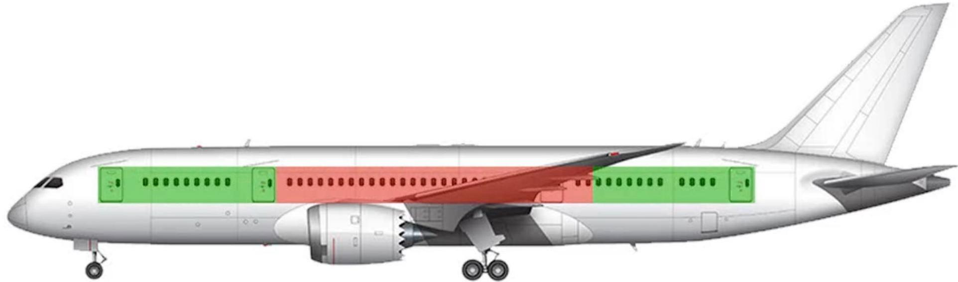
The **cut-in area** should be forward or aft of the wing.
