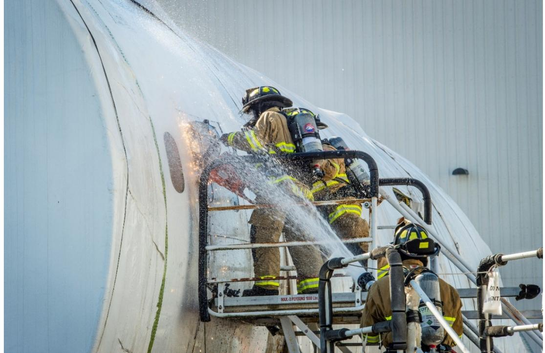
While performing cuts flow water from the crown of the aircraft over the cut area to limit particulates becoming airborne and to control sparking
