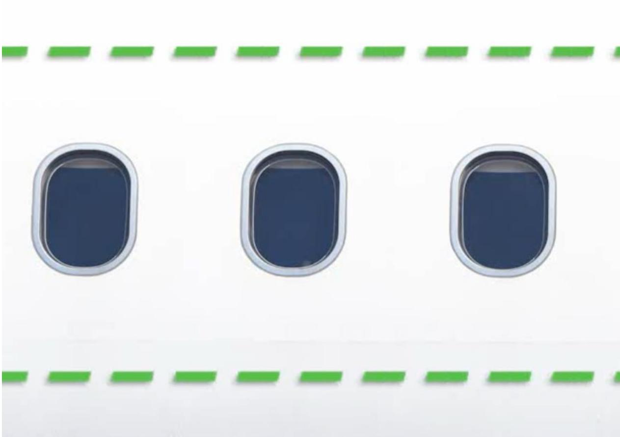
The recommend cut-in area is 12 inches (31 centimeters) above and 12 inches (31 centimeters) below windows.
