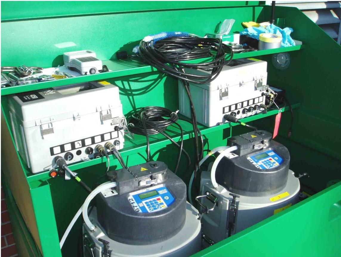
**Figure C-6. Double monitor setup for sampling over a wide range of flow conditions at Tuscaloosa, AL (Pitt, current projects)**
