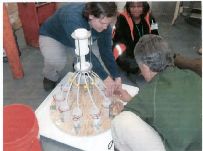
Expert Panel and MWH setting-up performance monitoring sample splitter, RWQCB observing.
