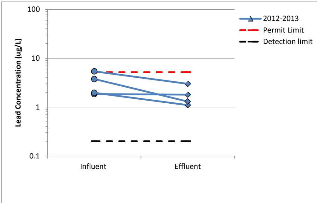
Figure 27. Lead at B1 Media Filter (CM), post curb cuts
