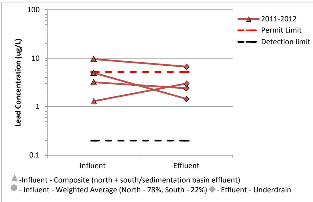
Figure 26. Lead at B1 Media Filter (CM), pre curb cuts
