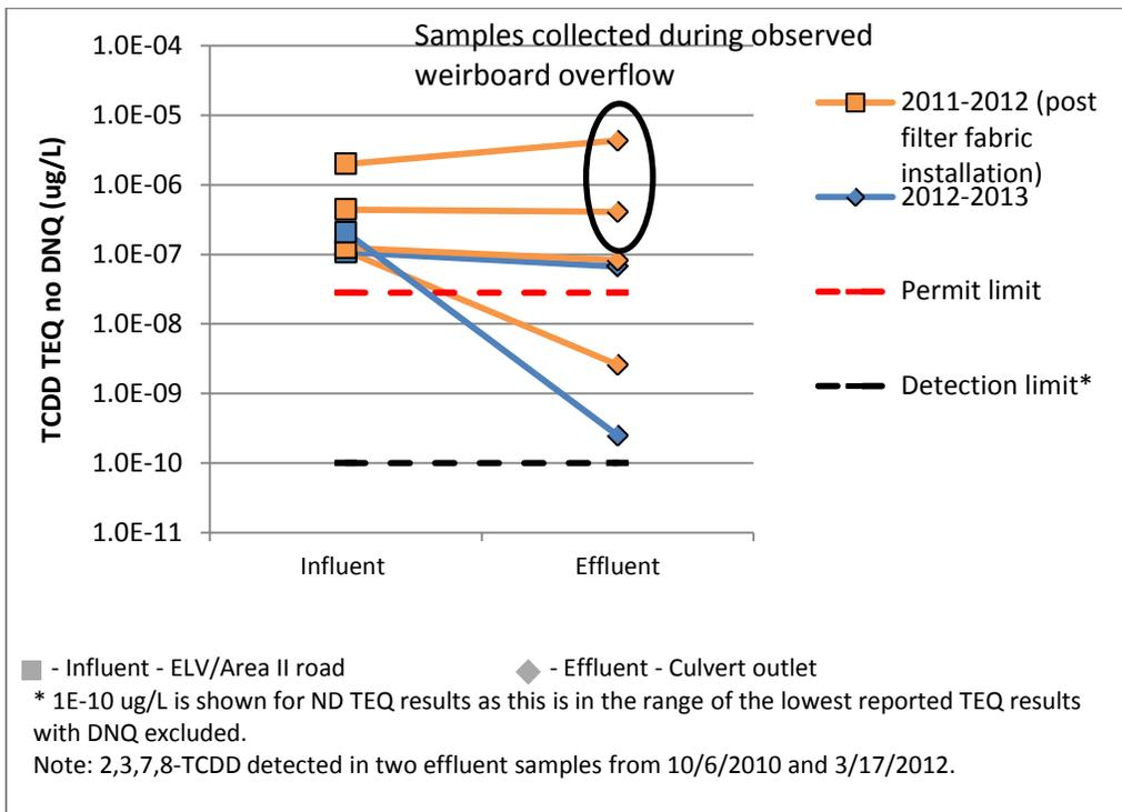
Figure 12. Dioxins at CM-1, post filter fabric installation
