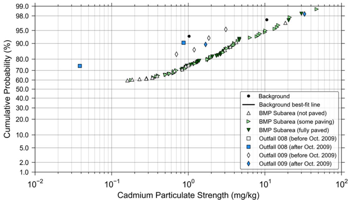
Figure 4. Probability plot for cadmium particulate strengths
