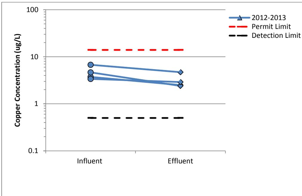
Figure 34. Copper at B1 Media Filter (CM), post curb cuts
