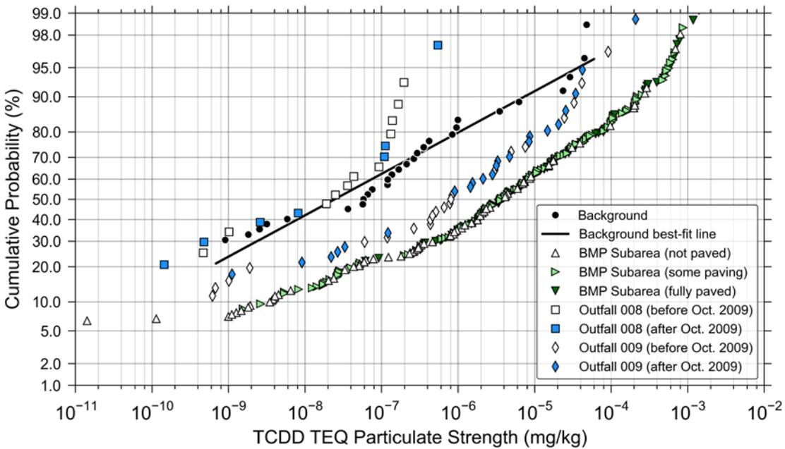
Figure 10. Probability plot for TCDD TEQ particulate strengths
