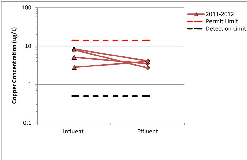
Figure 33. Copper at B1 Media Filter (CM), pre curb cuts
