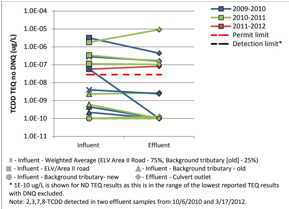
Figure 11. Dioxins at CM-1, pre filter fabric installation
