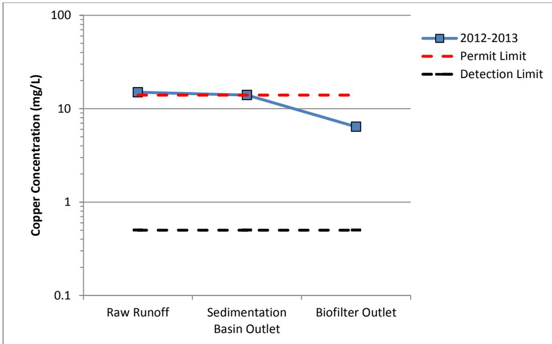
Figure 35. Copper at Lower Lot Biofilter, Watershed 009
