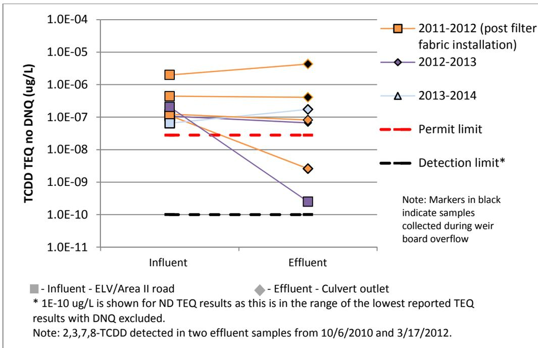
Figure 12. Dioxins at CM-1, post filter fabric installation
