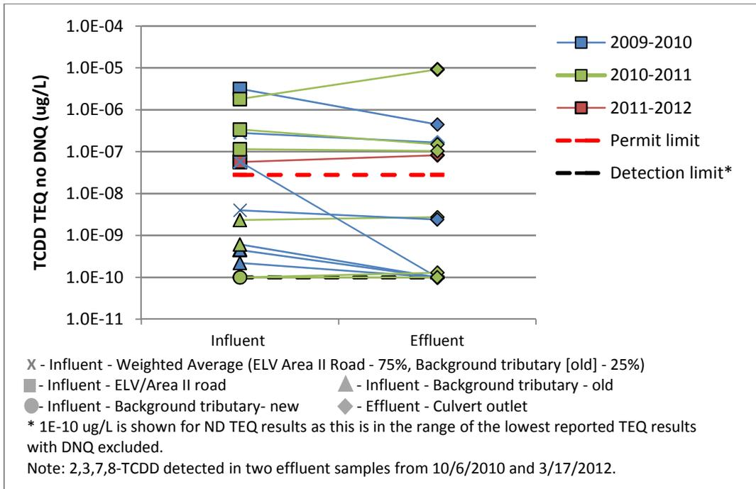
Figure 11. Dioxins at CM-1, pre filter fabric installation
