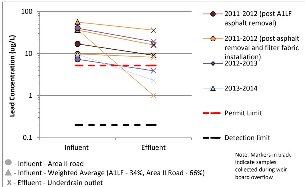
Figure 24. Lead at CM-9, post improvements (removal of A1LF asphalt and addition of CM weir board filter fabric)
