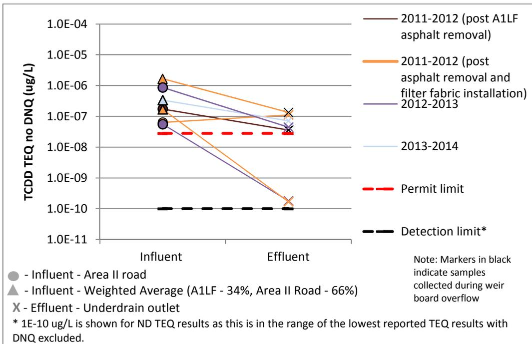
Figure 14. Dioxins at CM-9, post improvements (removal of A1LF asphalt and addition of CM weir board filter fabric)
