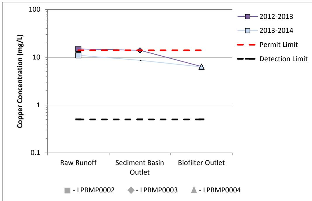
Figure 35. Copper at Lower Lot Biofilter<sup>7</sup>
