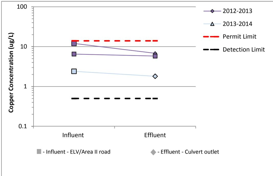
Figure 29. Copper at CM-1, post filter fabric installation
