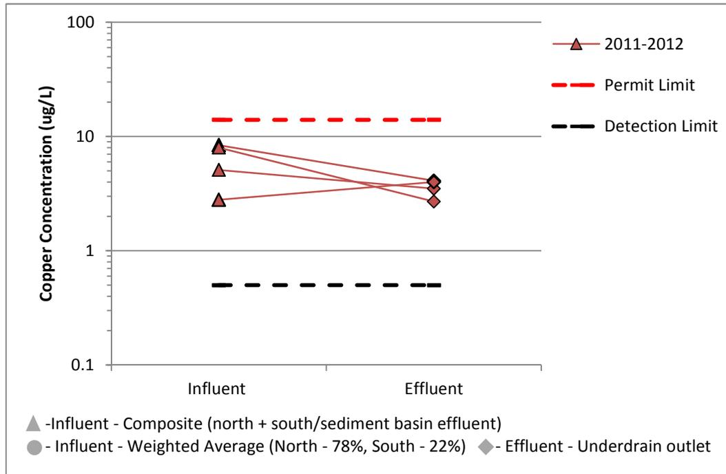
Figure 32. Copper at B1 Media Filter (CM), pre curb cuts
