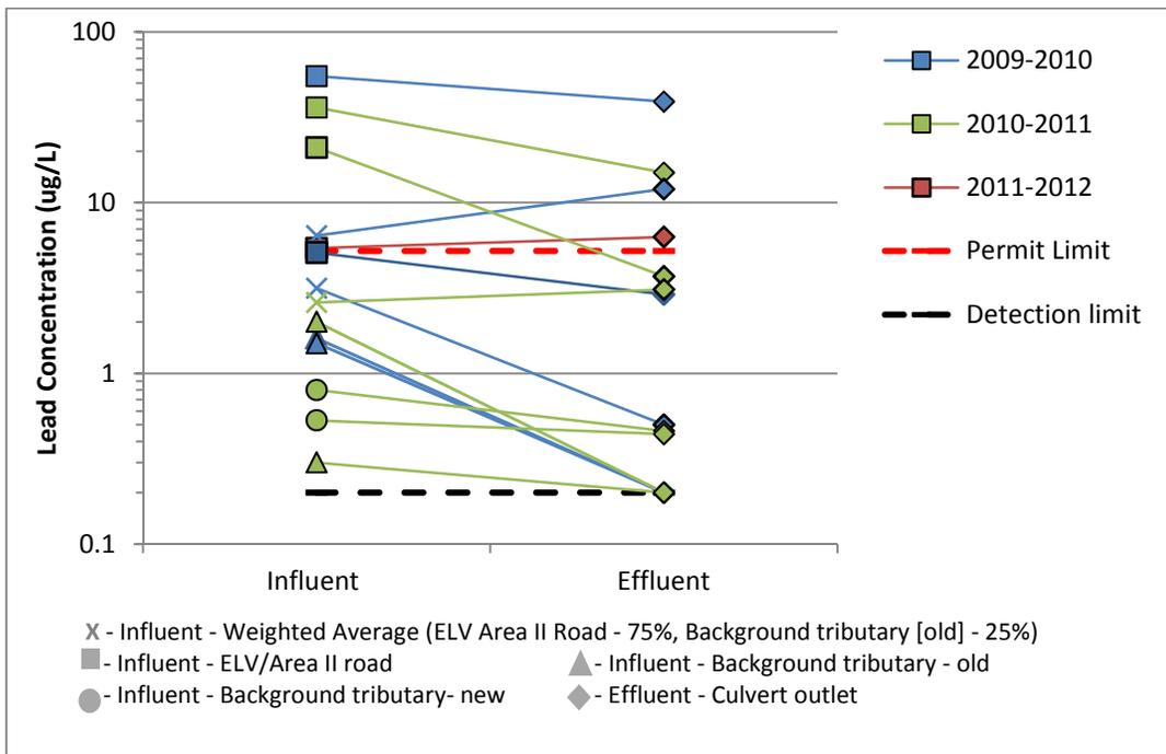
Figure 20. Lead at CM-1, pre filter fabric installation
