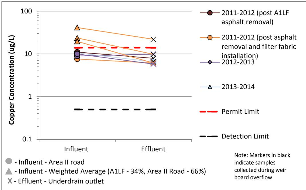
Figure 31. Copper at CM-9, post improvements (removal of A1LF asphalt and addition of CM weir board filter fabric)
