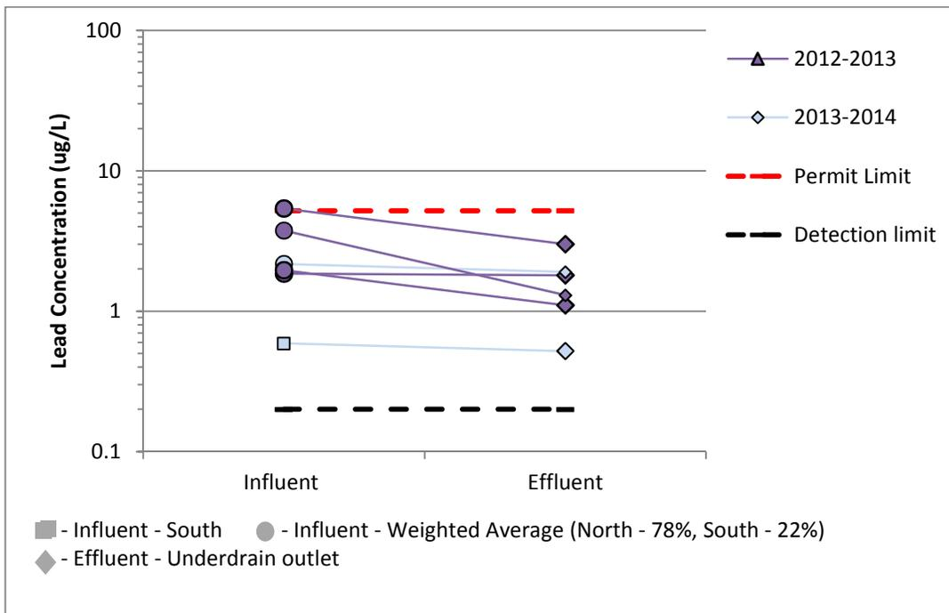
Figure 26. Lead at B1 Media Filter (CM), post curb cuts
