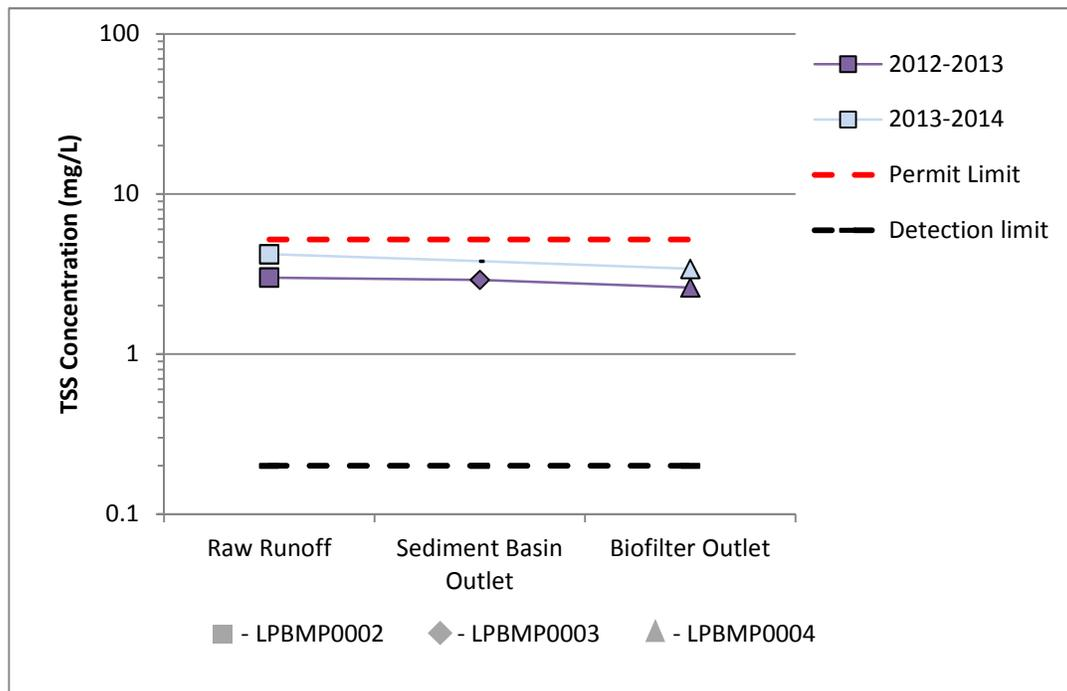
Figure 28. Lead at Lower Lot Biofilter<sup>7</sup>
