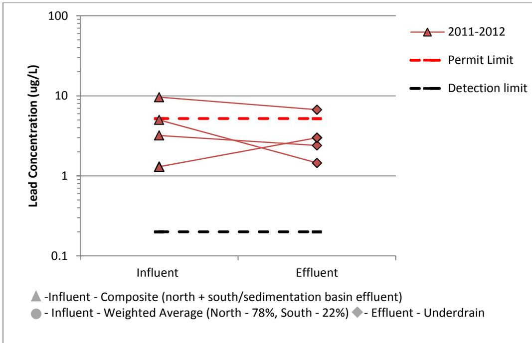
Figure 25. Lead at B1 Media Filter (CM), pre curb cuts
