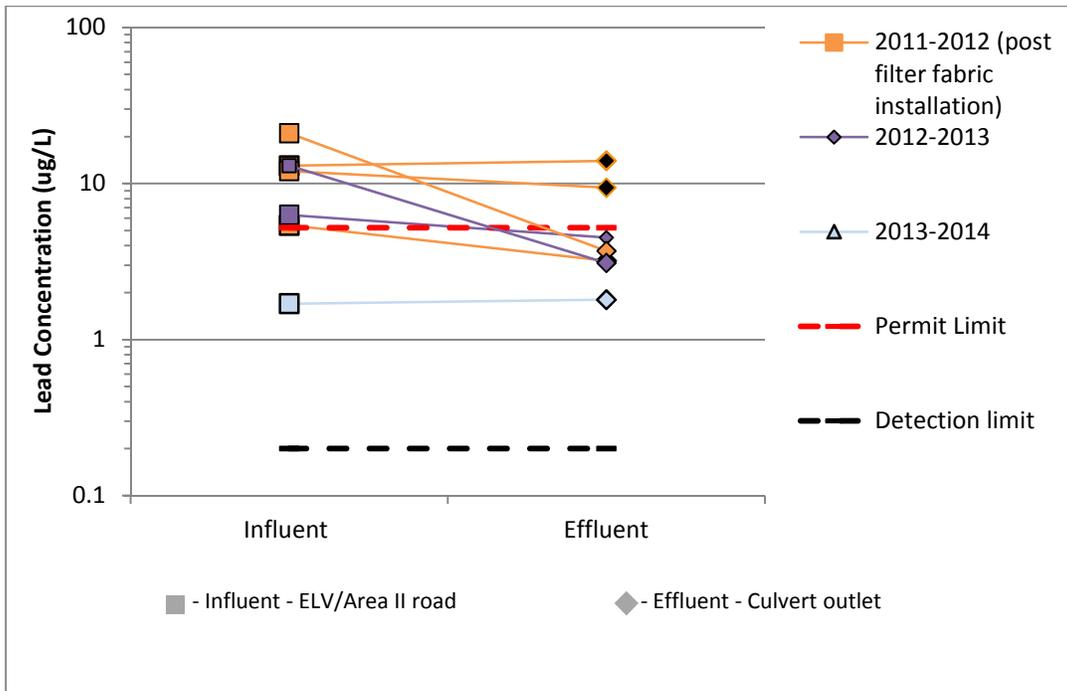
Figure 21. Lead at CM-1, post filter fabric installation
