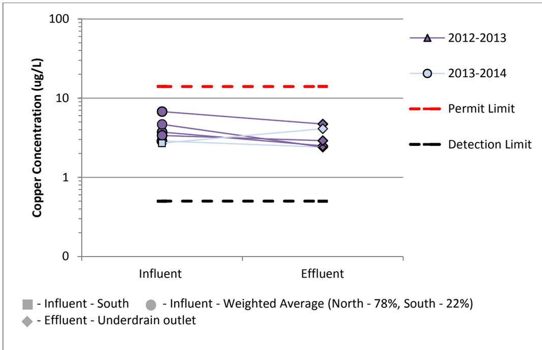
Figure 33. Copper at B1 Media Filter (CM), post curb cuts
