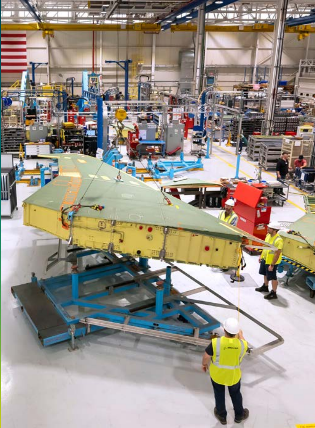
Teammates conduct a wing lift to move an F-15EX wing to the Final Assembly building in St. Louis.
