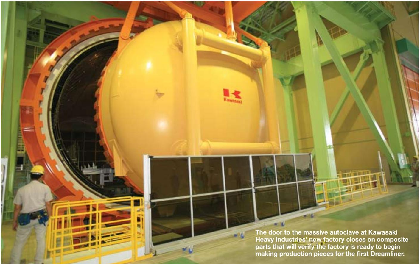
The door to the massive autoclave at Kawasaki Heavy Industries' new factory closes on composite parts that will verify the factory is ready to begin making production pieces for the first Dreamliner.
