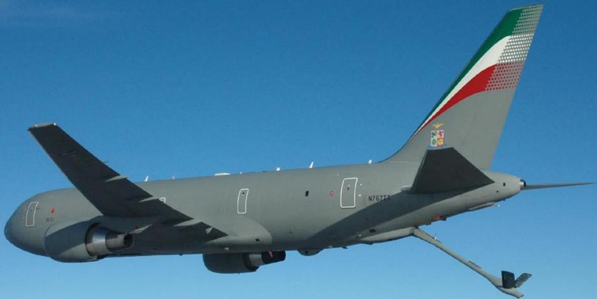
**In late September, the KC-767 Tanker deployed its fly-by-wire boom for the first time during flight. The milestone demonstrates integration between the aircrew operator and the advanced refueling system.**
