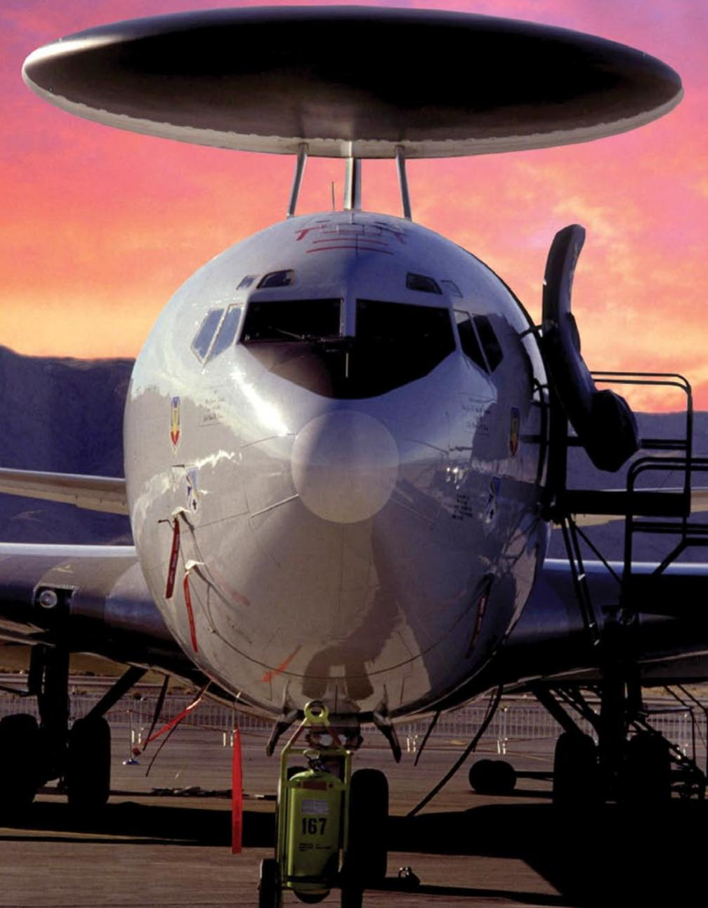
This head-on view of the E-3 Sentry shows its distinct rotodome. Measuring 30 feet wide and 6 feet thick (9.1 by 1.8 meters), it scans at six revolutions per minute. When not in operation, it continues to rotate once every four minutes.
