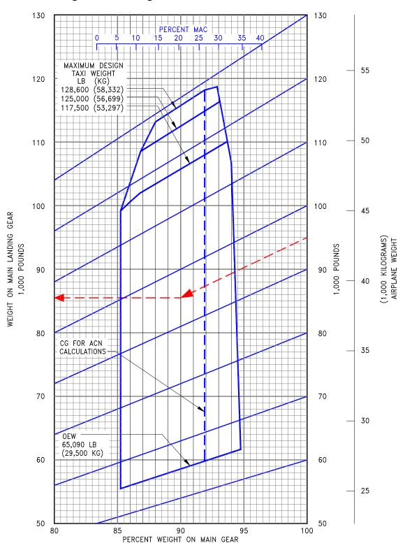
7.4.3 Landing Gear Loading on Pavement: Model 737-200 Advanced
