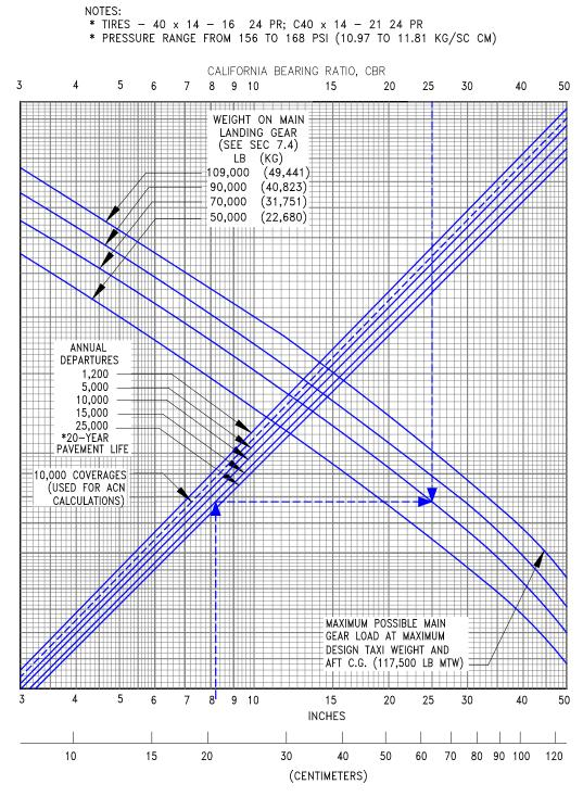
FLEXIBLE PAVEMENT THICKNESS, h
