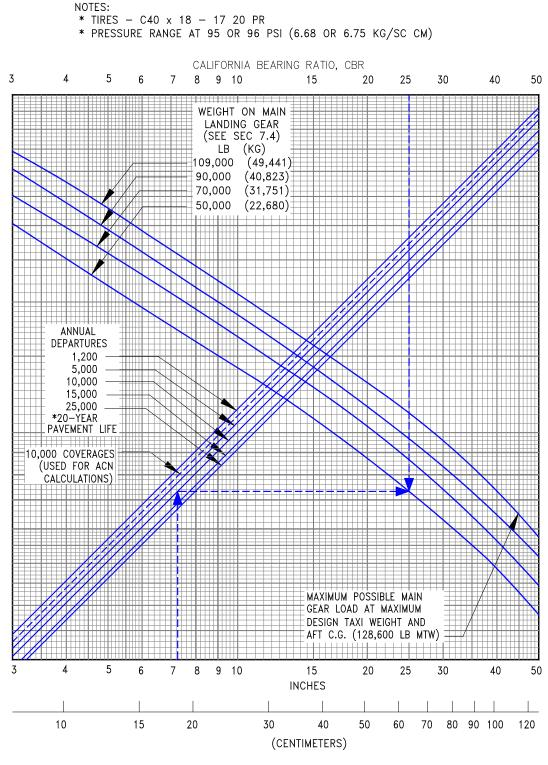
FLEXIBLE PAVEMENT THICKNESS, h
