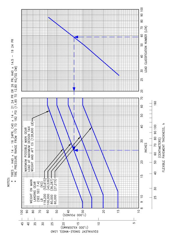
7.6.4 Flexible Pavement Requirements - LCN Method: Model 737-200 ADV at 120,000 to 128,600 LB (54,431 to 58,332 KG) MTW
