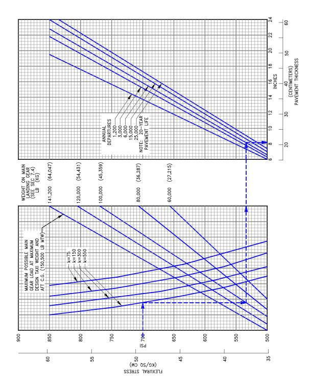
7.9.3 Rigid Pavement Requirements – FAA Design Method: Model 737-300, -400, -500
