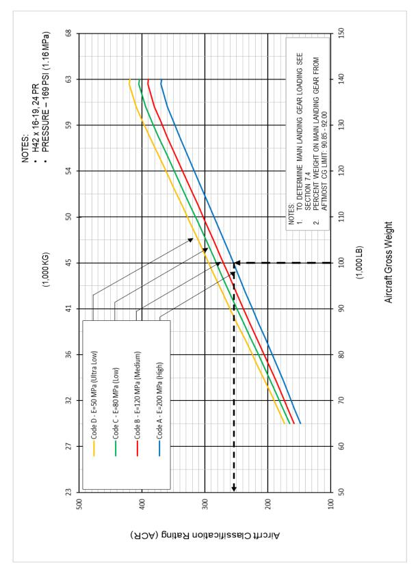
7.11.14 Aircraft Classification Rating – Rigid Pavement: Model 737-300 Low Tire Pressure
