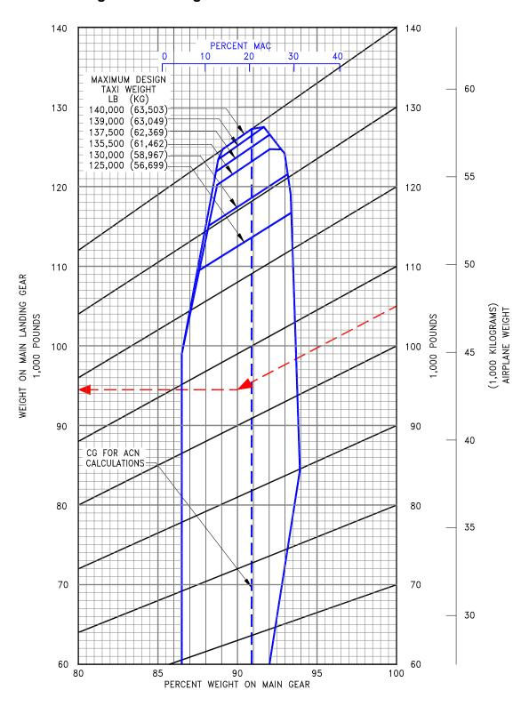
7.4.4 Landing Gear Loading on Pavement: Model 737-300
