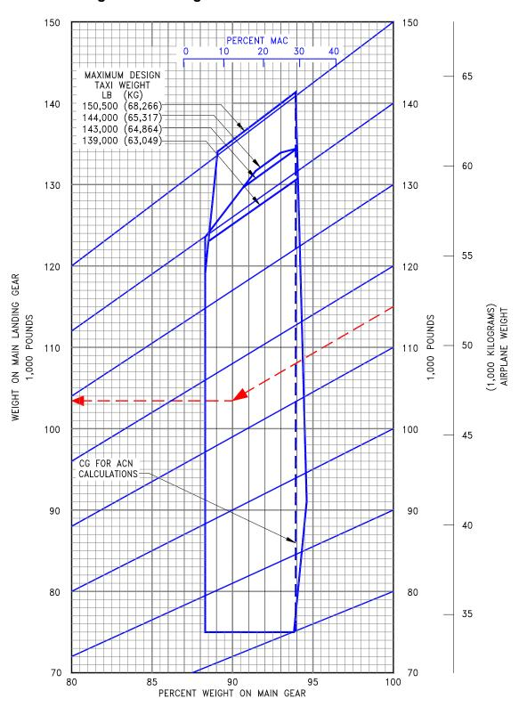
7.4.5 Landing Gear Loading on Pavement: Model 737-400
