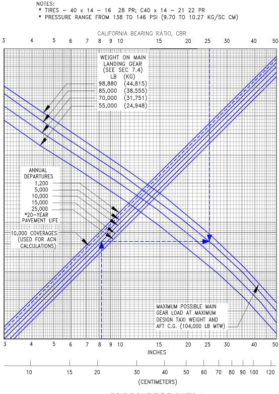
FLEXIBLE PAVEMENT THICKNESS, h
