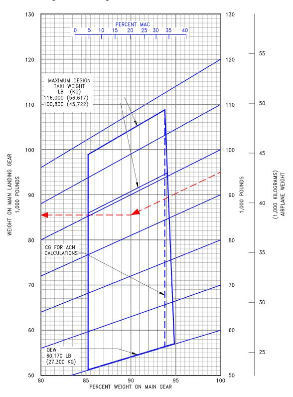
7.4.2 Landing Gear Loading on Pavement: Model 737-200
