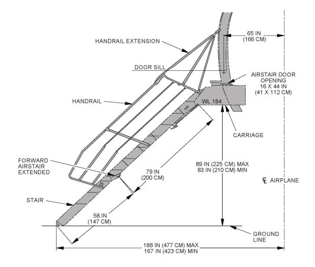
2.7.4 Door Clearances: Sensor and Probe Locations - Forward Cabin Doors: All Models
