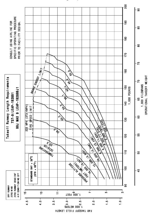
3.3.24 FAA/EASA Takeoff Runway Length Requirements - Standard Day + 63°F (STD + 35 °C), Dry Runway: Model 737-9 / BBJ MAX 9 (LEAP-1B28 / LEAP-1B28BBJ1 Engines)
