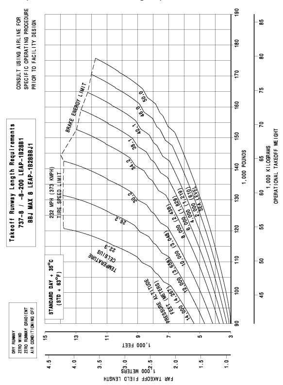
3.3.16 FAA/EASA Takeoff Runway Length Requirements - Standard Day + 63°F (STD + 35 °C), Dry Runway: Model 737-8 / -8-200 / BBJ MAX 8 (LEAP-1B28B1 / -1B28BBJ1 Engines)
