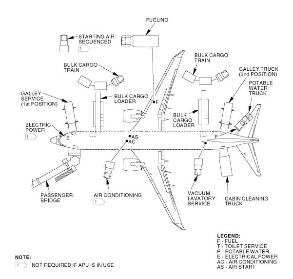
5.1.3 Airplane Servicing Arrangement - Typical Turnaround: Model 737-9 / BBJ MAX 9
