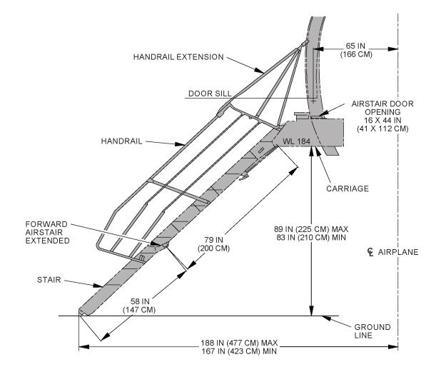
D6-38A004 March 2023 2.7.4 Door Clearances: Sensor and Probe Locations - Forward Cabin Doors: All Models
