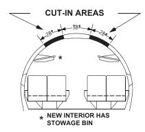
NOTE: CUT-IN AREAS REQUIRE METAL CUTTING PORTABLE POWER EQUIPMENT. BECAUSE OF TYPE OF STRUCTURE AND POSSIBLE INJURY TO PERSONNEL WITHIN, IT IS RECOMMENDED THAT MAJOR EFFORT TO GAIN ACCESS BE DIRECTED TO HATCHES AND DOORS. URGENCY OF SITUATION WILL DICTATE THE
