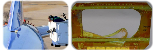
Figure 3. Example of an in-service structural failure used for an inductive learning approach to fatigue cracking and the merits of fail-safe design [10].
