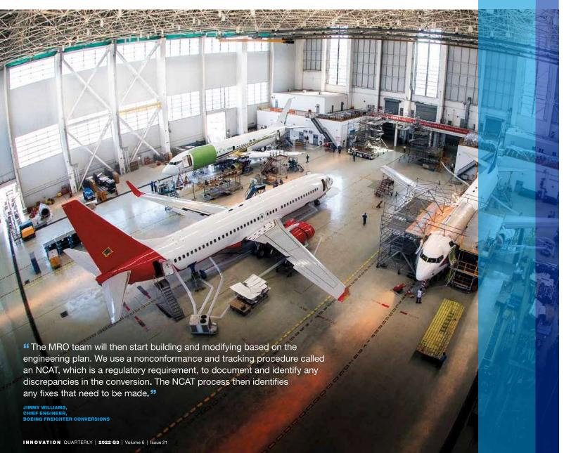
"The MRO team will then start building and modifying based on the engineering plan," said Williams. "We use a nonconformance and tracking procedure called an NCAT [nonconformance corrective action tool], which is a regulatory requirement, to document and identify any discrepancies in the conversion. The NCAT process then identifies any fixes that need to be made."
