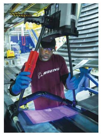
New capabilities were tested and incorporated into the production process to verify skin flatness conformance following the fabrication of the fuselage section. The team adapted a tool, originally developed in the automotive industry, as a shop aid to identify areas where the join surface potentially didn't meet flatness requirements. Following the final preparation of the fuselage join surface, a laser scanner is now used to confirm conformance to design specifications.
