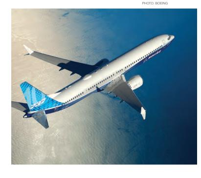
The 737 MAX improved on Next-Generation 737 range with the capability to fly more than 3,500 nautical miles (6,510 km), an increase of 340-570 nmi (629-1,055 km). The 737 MAX also incorporates quiet engine technology to reduce the operational noise footprint of the airplane by up to 40 percent.
