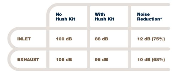
\* Noise is measured in decibels (dB) on a logarithmic scale. For every 6 dB reduction, the actual noise is cut in half. -Noise is generated by the ECS, which operates during the electronic testing phase for the AH-64 Apache. - Measurements were collected at the source with a calibrated CEL-254 sound level meter, in accordance with OSHA standards for instrumentation to measure exposure to noise.
