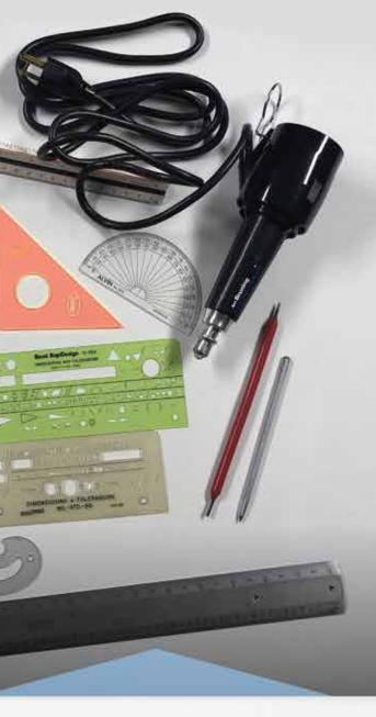
The red and gray tools on the right were used for drawings on vinyl film. The ink pens and black electric eraser applied or removed ink on polyester film.
