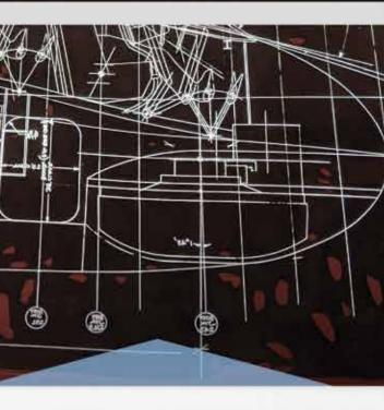
On the back side of polyester film, red paint was used to block out any pinholes or errors that let light through.
