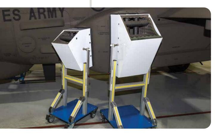
Third, each unit needed to gimbal in all axes (x, y and z). This was vital because the seal needs to fit tightly to the aircraft in order for the sound suppression to work well. Axes x and y were dealt with using swivel bearings attaching the hush box to the frame. Casters on each corner of the base plate took care of the z axis.
