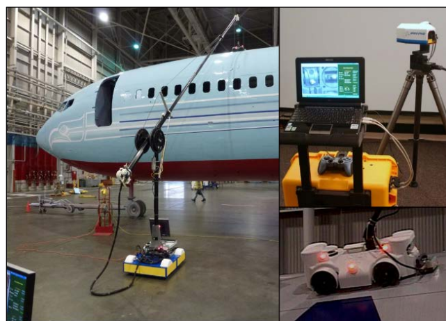
Figure 10. Boeing ROVER (Remotely Operated Vacuum Enabled Robot) for aircraft (and other) exterior structural NDE. In the left photo the system is shown during an inspection demonstration, with the mobile automated boom that provides fall protection, power, and communication to the crawler, which is shown in the lower left photo. The LPS (shown in the upper right photo) is one method that is used for guidance and tracking of the crawler.
