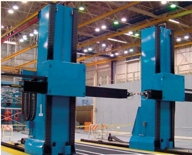
Figure 5a. Boeing AUSS Tower, used for NDE of large composite structure during manufacturing.
