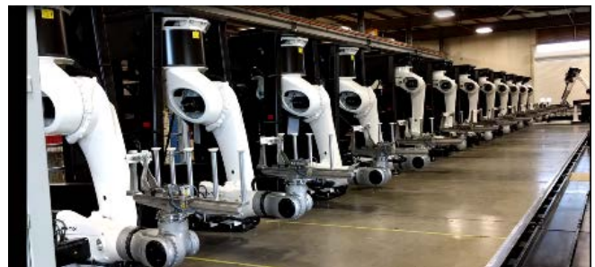
Figure 6. 777X Wing spar Robotic NDE Cell. The row of robots on the left hold and spar, while the robot on the right inspects it.
