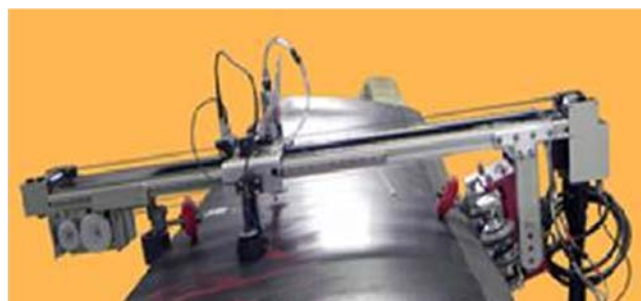
Figure 11. The Boeing Blade Crawler is shown traversing a helicopter rotorblade during an inspection.
