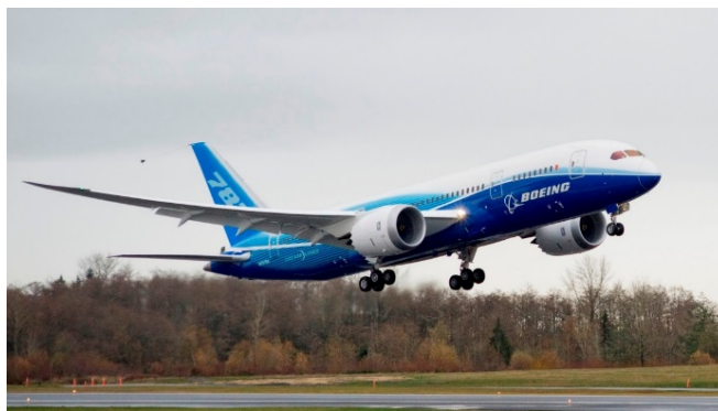
Figure 4. Boeing 787 Dreamliner, whose structure is just over 50% composite by weight.
