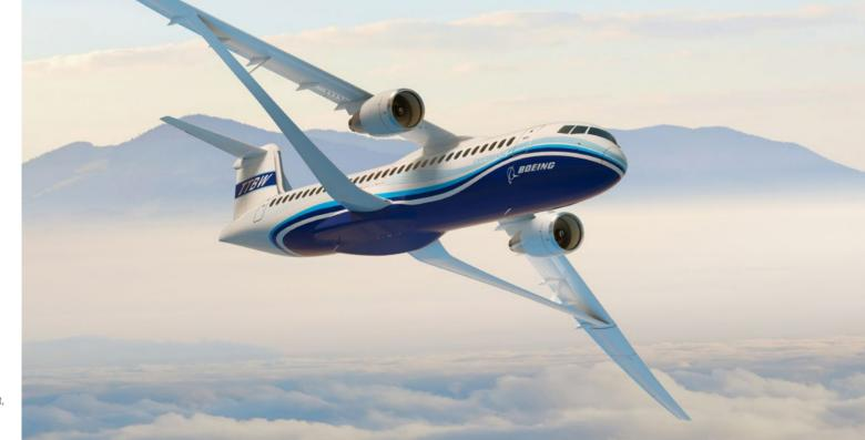
Boeing is studying the Transonic Truss-Braced Wing concept, designed to be more aerodynamic and fuel efficient, through a collaboration with NASA as part of the Subsonic Ultra Green Aircraft Research program. (Boeing illustration)
