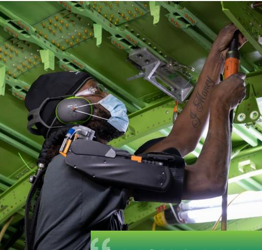
Working on a 767 in Everett, Washington, mechanic Jason Turner is much more comfortable thanks to a shoulder support exoskeleton. (Boeing photo) By enhancing Boeing's safety culture through risk reduction, creating a safe work environment and ensuring productive processes and interactions, all employees can leave work as safely as they arrived."
