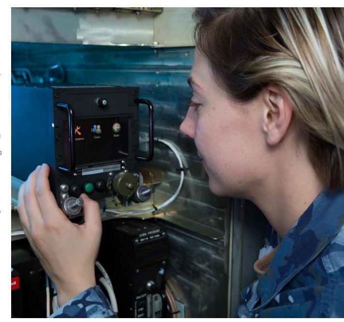
An aviator with the Royal Australian Air Force performs system checks on a C-17 with Boeing's Aircraft Data Reasoner. (RAAF photo)
