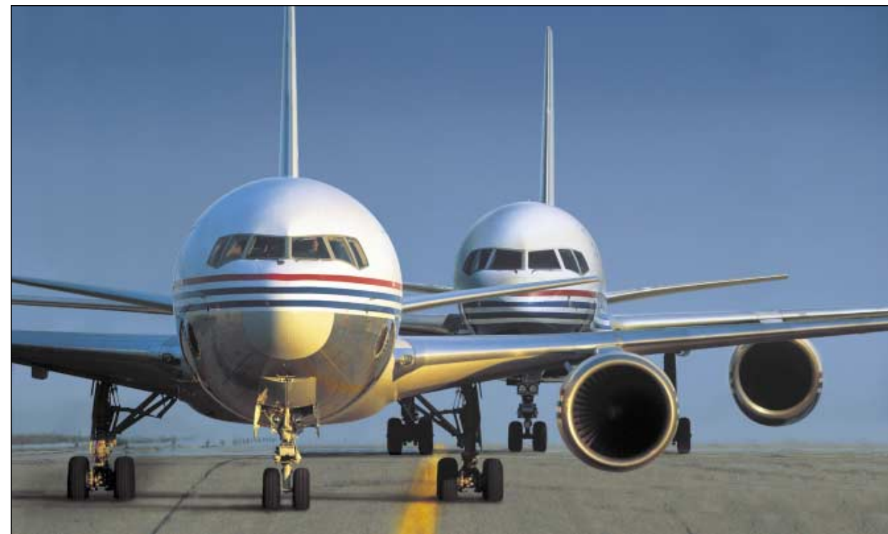
The 767, left, is shown with its sibling airplane, the 757. The planes were developed at the same time and are the only two Boeing commercial airplanes to offer flight deck joint certification.
