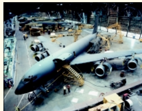
Boeing in Wichita has a rich history and promising future in tankers. Here employees perform a re-engineing program on a KC-135R.
